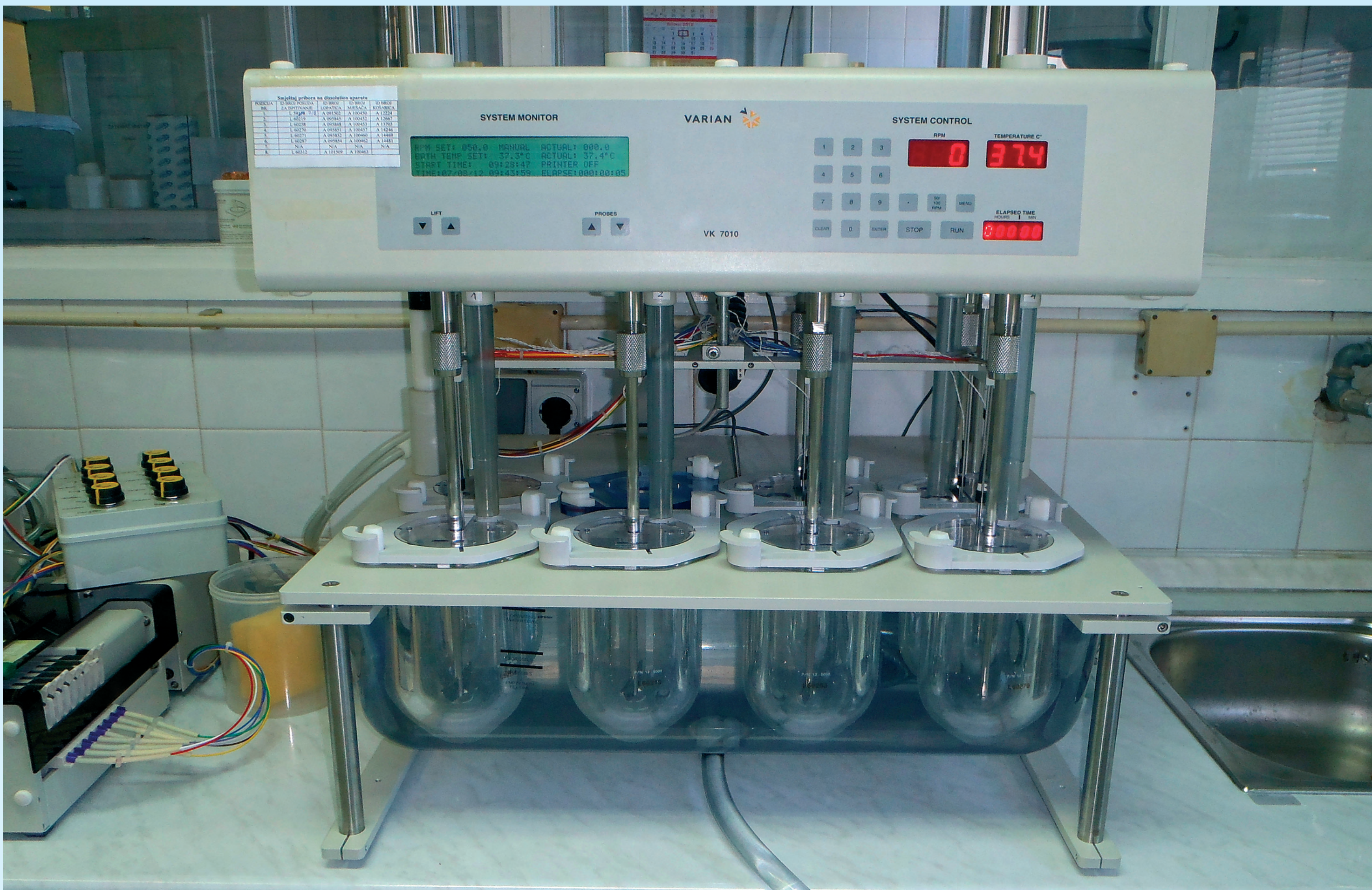
Picture 1: All folic acid dissolution tests were carried out by Varian VK 7010 dissolution apparatus
