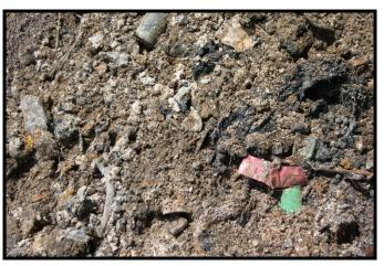
Photo: Three of the seven test trenches identified buried solid waste. Solid waste included pieces of concrete, rusty metal, glass bottles, broken glass, metal cans, and plastic.
